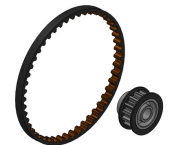
The drive pulley is equipped with 18T as standard. Option 15T (Pulley & Belt Set for low gear) set. For the primary reduction ratio, 2.11 for 38T - 18T and 2.53 for 38T - 15T can be selected.
