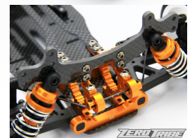
Body post for using the narrow roof body can be mounted on the rear side damper stay.
