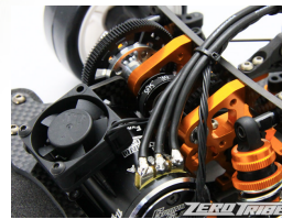
The drive pulley is equipped with 18T as standard. Option 15T (Pulley & Belt Set for low gear) set. For the primary reduction ratio, 2.11 for 38T - 18T and 2.53 for 38T - 15T can be selected.
