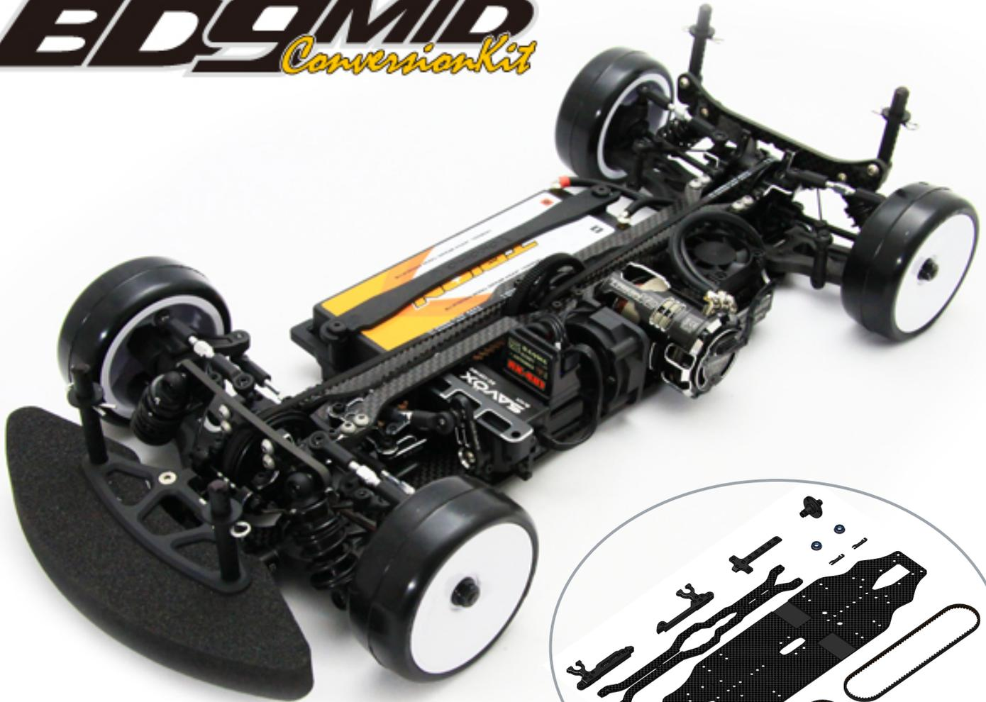
This product is a conversion kit based on the YOKOMO BD9. The purpose of development is to reduce the time lag at the time of throttle operation as much as possible by eliminating the difference in belt length between front and back. As a result, the motor is laid out on the center side, enabling a balanced midship layout to be realized.
