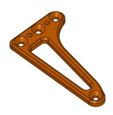
This product is a floating servo holder for XRAY T4 '17' 18. 7075T6 is used for the material of this product. The ambiguity at the beginning of the steering operation disappears and it becomes sharp handling. The weight is about 5.4 g. The color of the alumite is orange.
