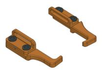
This adjustable battery holder for XRAY T4 is made from A7075 extra-super duralumin. With the pitch about 1mm on both the right and left sides, it can be adjusted in three steps. It moves freely longitudinally along the groove. The glass tape holder can be used with or without the side guard.
